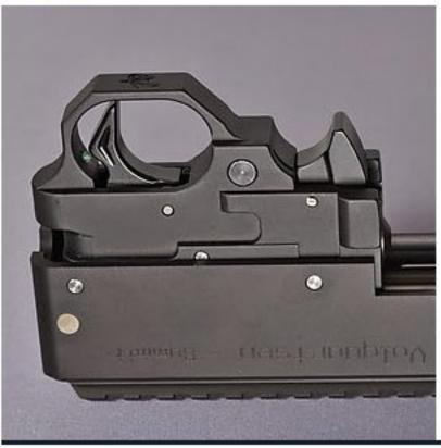
Insert the trigger group into the receiver and install pins to hold it in place.
