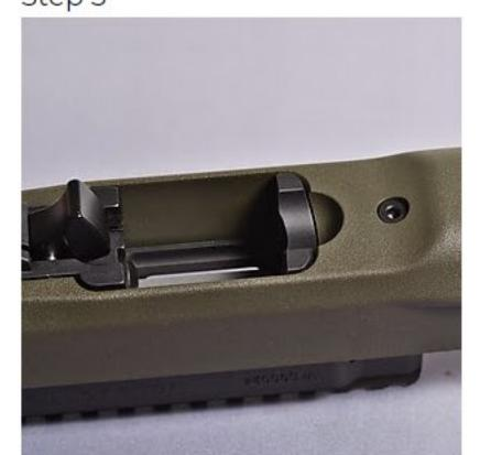
Install the barreled action in the stock, being careful to ensure that the pins holding the trigger group do not fall out.
