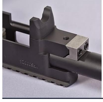
Use the 12-24 screws and V-Locking Block to secure the barrel to the receiver. Be sure that the V-Locking Block is flush with the receiver and not tilted to once side or the other.
