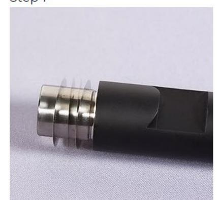
Setting proper headspace is critical to the function and safety of the Summit Action. Start by placing four shims over the shank of the barrel in preparation for inserting it into the receiver.
